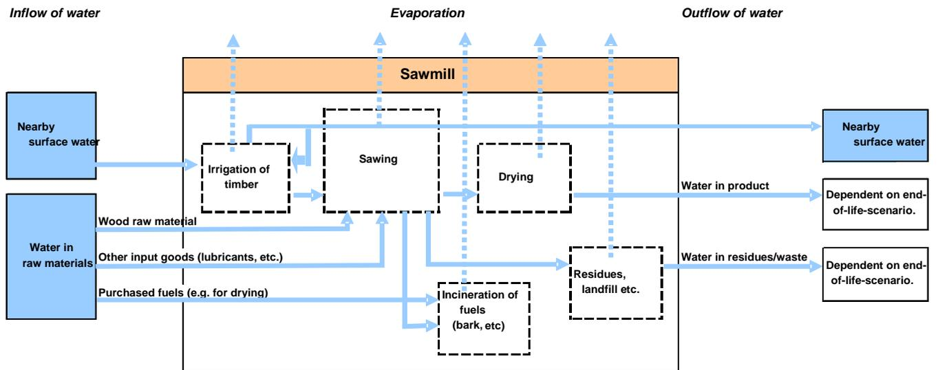
**Figure 8.** Schematic diagram of water flows included in the manufacture of sawn timber.
