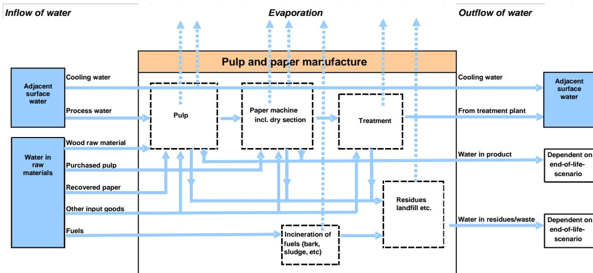
**Figure 7.** Schematic diagram of water flows included in the manufacture of pulp and paper products.
